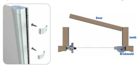
You may choose to position the screen inside the door frame in one of the locations shown below. Typically the handle on the door does not affect the screen placement decision. This is because the door will be open while the screen is being used and the screen will be retracted when the door is closed.
